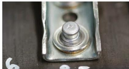
Clearly visible piston mark on top washer
