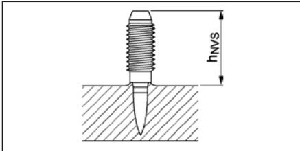
X-ST-GR M8/5 P8,  $h_{NVS} = 12.0-15.0 \text{ mm}$
