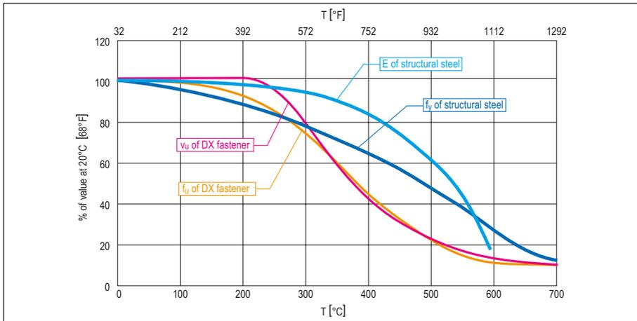
Up to about 300°C [572°F], the strength loss for DX fasteners is roughly proportional to the yield strength loss of structural steel. At 600°C [1112°F], DX fasteners have about 12% of their 20°C [68°F] strength left and structural steel about 26%. Since DX fasteners obtain their high strength through a thermal hardening process, the loss in strength at elevated temperatures is proportionally greater than for structural steel.
