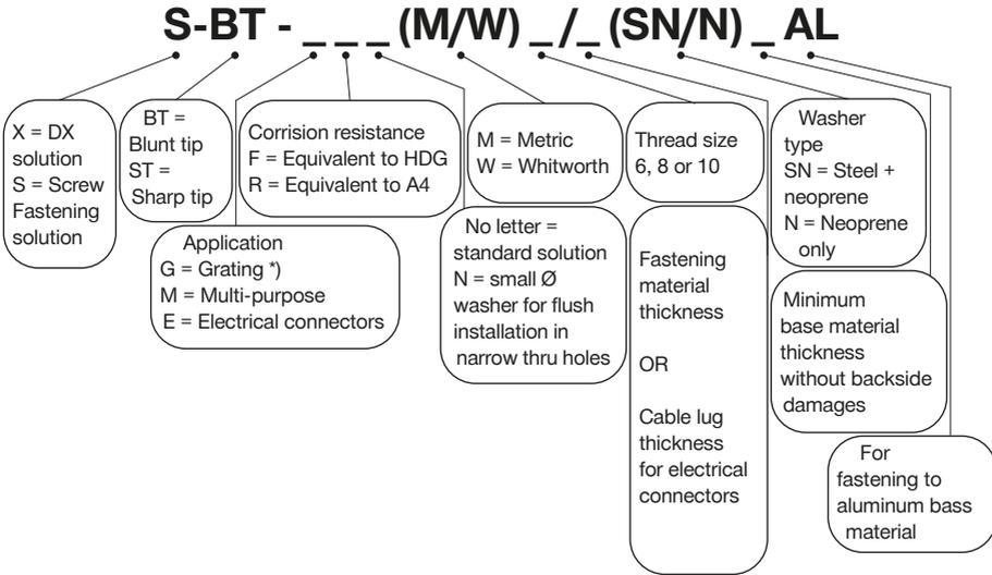
\*) X-ST-GR stainless steel threaded studs may also be used for multi-purpose applications.
