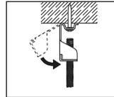
5. Bend the X-HS assembly down to the vertical position
