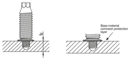
\*) for the applications "Functional bonding and terminal connection in a circuit" and "Protective bonding circuit" the minimum base material thicknesses can be reduced to  $t_{II} = 3 \text{ mm}$ . Applicable only for Type A, single point connections.
