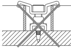
The saddle of the fastener should not be bent, see installation instruction above.
