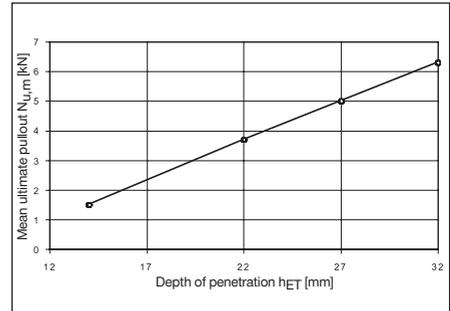
The value of increasing the depth of penetration in order to increase pull-out strength is limited by the increasing fastener driving failure rate. Provided that the penetration depth is the same, fastenings in concrete with a higher compressive strength hold better than fastenings in lower strength concrete. The ability to exploit this
