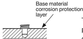
Thickness of base material corrosion protection layer  $\leq 0.4\text{mm}$ . For thicker coatings, please contact Hilti.
