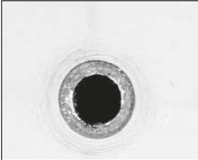
Pre-drill with TX-PGR-RU-4/10-93 step shank drill bit (Item no. 2061802), until shoulder grinds a shiny ring (to ensure proper drilling depth).
