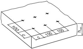
Base material thickness:  $h_{\min} = 80 \text{ mm}$
