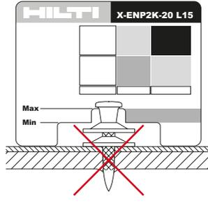
$h_{NVS} > 11 \text{ mm}$
