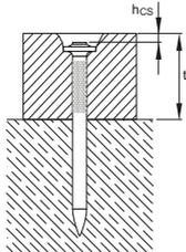
X-GN 39:  $h_{CS} = 2-3$  mmFastening to steel
