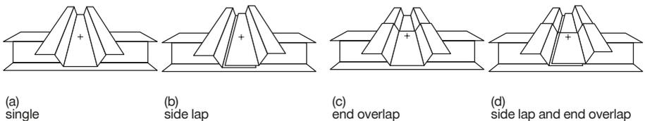
As part of a steel deck diaphragm, all four fastening types (a), (b), (c) and (d) are executed with the X-HSN 24, X-EDNK22 and the X-EDN19. The sheet metal thickness typically varies between 22 Gauge (0.76 mm) and 16 Gauge (1.52 mm).
