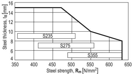
Application limit may increase in case of specific applications, like the fastening of wire mesh to steel, which is connected with X-CC U16 P8 fasteners. That wire mesh acts as reinforcement for fire protective sprayed coating. In such cases also different fastener stand-offs apply. Inquire at Hilti related with the use of X-CC U16 P8 in that specific application.
