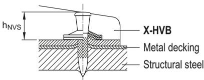
$$8.2 \text{ mm} \leq h_{NVS} \leq 9.8 \text{ mm}$$
