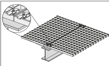
For fastenings exposed to weather and mildly corrosive conditions.
