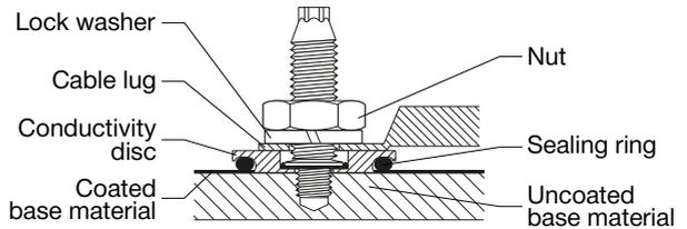
For Type B cable connection the following requirements have to be observed:
