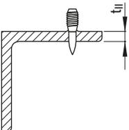
Steel thickness:  $t_{II} \geq 6 \text{ mm}$
