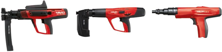
These tools rely on cartridges of different power levels as propellant. When ignited, the cartridge transfers energy to a piston which, in turn, drives the fastener into the base material.
