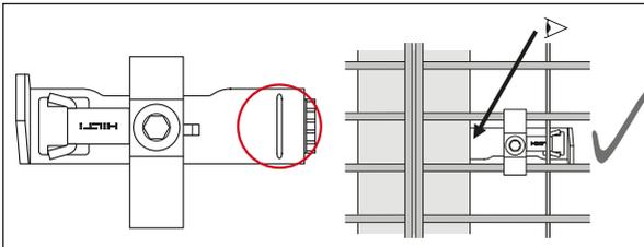
The sign on the clip has to be positioned under the steel flange
