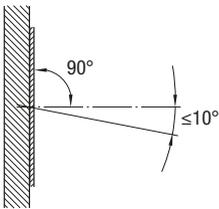
Position the DX tool so that nail inclination is limited to max. 10° from perpendicular to surface
