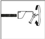
1. Attach the threaded rod to the X-HS before fastening
