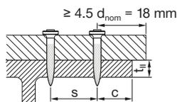
Base material thickness:  $t_{II} \geq 6.0 \text{ mm}$
