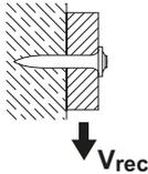
Fastening wood to concrete, sandlime masonry:
