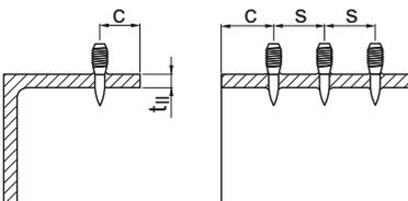
$$\text{Edge distance: } c \geq 15 \text{ mm}$$
