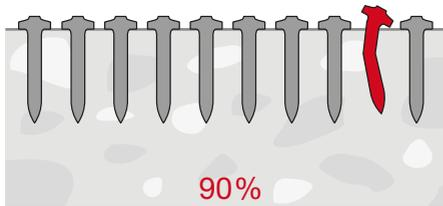
The stick rate indicates the percentage of nails that are driven correctly to carry a load.
