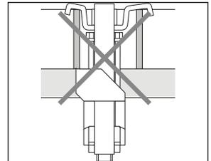
The saddle of the fastener should not be bent, see installation instructions below.
