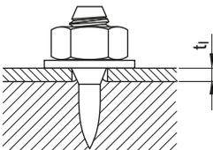
$$t_I \leq L_g - t_{\text{washer}} - t_{\text{nut}}$$
