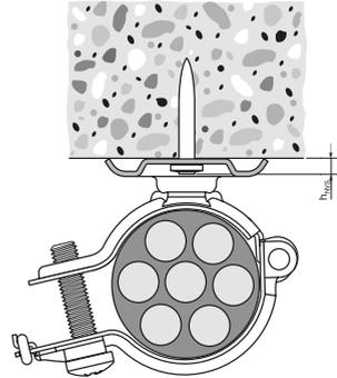
$$h_{NVS, \min} = 3 \text{ mm}$$
