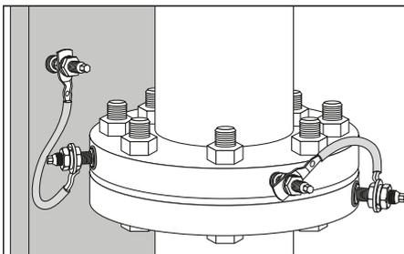
Functional and protective bonding of pipes \*)
