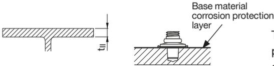
Thickness of base material corrosion protection layer  $\leq 0.4$  mm. For thicker coatings, please contact Hilti.
