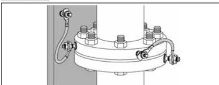
Functional and protective bonding in pipe
