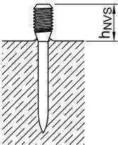
$$h_{NVS} = L - h_{ET}, \quad h_{ET} = 37-41 \text{ mm}$$
