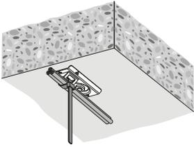
Fastening electrical installation to ceiling and wall
