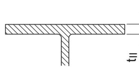
$t_{II} \geq 4.0 \text{ mm}$  (for nail)
