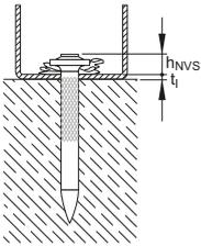
X-GN/GHP:  $h_{NVS} = 2-5$  mm
