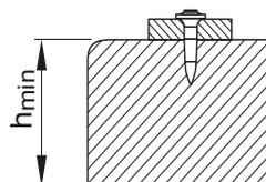
Concrete:  $h_{min} = 80 \text{ mm}$
