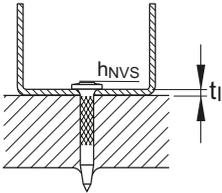
X-S:  $h_{NVS} = 2-4 \text{ mm}$
