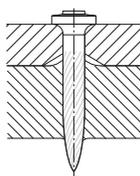
If a gap between the fastened part and the base material is unacceptable, the fastened part needs to be prepared with drilled holes.
