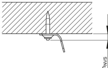
$$h_{NVS, \min} = 6 \text{ mm}$$
