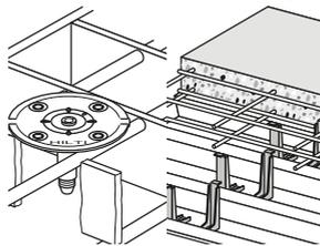
The nails used (also known as drive pins) are of a special type equipped with washers to meet the needs of the application and to provide guidance when driven. Threaded studs are essentially nails with a threaded upper section instead of a head. Composite fasteners are an assembly consisting of a nail with an application-specific fastening component such as a clip, plate or disk made of metal or plastic.
