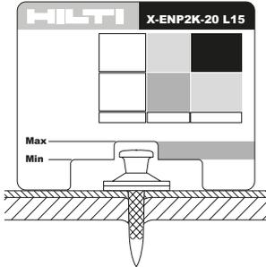
$h_{NVS} = 7-11 \text{ mm}$
