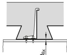
Maximum total thickness of fixed sheeting  $t_{fix}$ :
