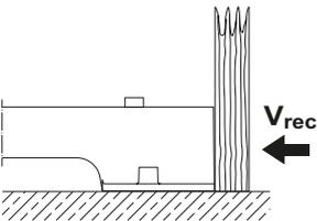
Shear load:  $V_{rec} = 0.4 \text{ kN}$
