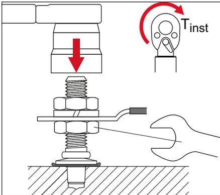
Hold the bottom nut with a spanner while tightening the upper nut.
