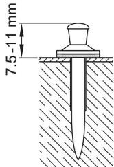
Check for conformity with recommendations (detailing spacing and edge distances for fastening)
