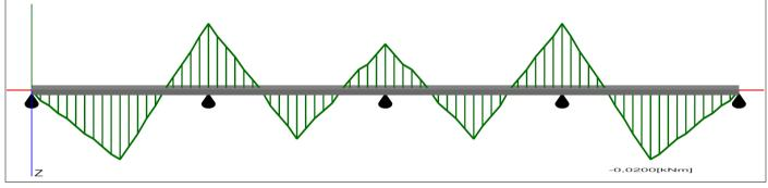
Deflection (Load combination Z: LC2-SLS Y: LC2-SLS )
