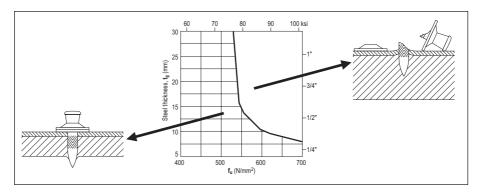
The application limit lines for long nails used to fasten wood to steel are plots of nail shank length  $L_{\rm S}$  versus steel thickness  $t_{\rm II}$ . Each line is valid only for one ultimate tensile strength of steel  $f_{\rm u}$ . Attempts at working to the right of the limit line result in buckled nail shanks.
