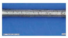
Suitable stainless steel used, e.g. HCR material used in a road tunnel
