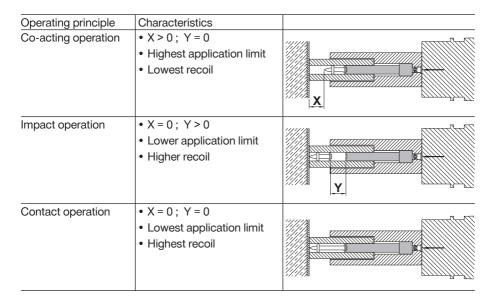
It should be noted that 100% co-acting operation in Hilti tools can be only achieved by pushing the fastener all the way against the piston with a ramrod or, if the tool is so designed, with a built-in ramrod mechanism. Tools with nail magazines cannot operate with 100% co-action because of the need for clearance between the piston end and the collated nail strip. Some single-shot tools allow the operator to make an impact-type tool work as a co-acting tool by using a ramrod.
