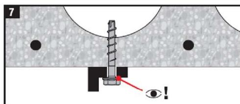
Installation with other electrical impact screw drivers of equivalent force and performance is possible.
