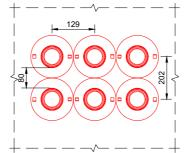
Zero Distance between Devices - For Double Gangplate installation: (200mm from one Double Gangplate to another Double Gangplate)
