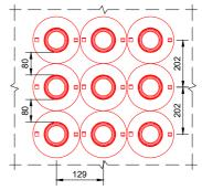
Zero Distance between Devices (200mm from one Triple Gangplate to another Triple Gangplate)
