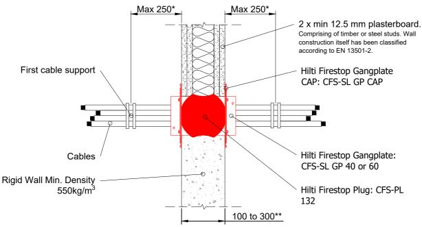
Depending on Fire Classification and space requirements, the Hilti Firestop Sleeve CFS-SL GP can be installed with: ≥ 200mm distance between openings, or Gangplates touching or slight overlap (zero distance)
